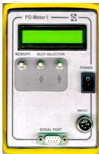
Fig. 2 Digital slot discharge meter with storage capabilities
