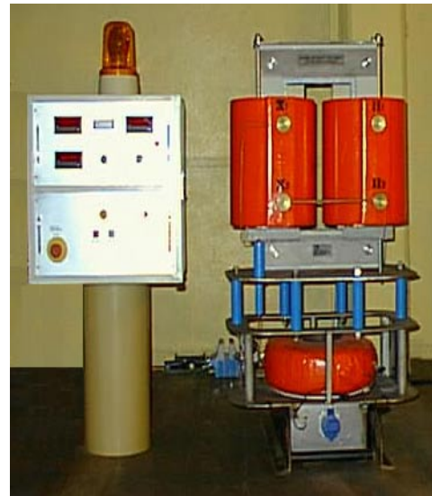
Fig. 1 Variable frequency resonant transformer
