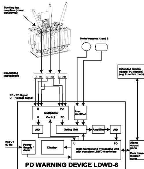
Figure 12: Block diagram of the PD monitoring system for power transformers
