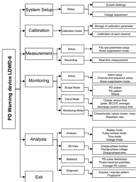
Figure 11: Software concept of the PD monitoring system
