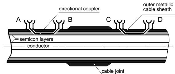
Figure 4b: Principle set-up of two sensors at a cable joint
