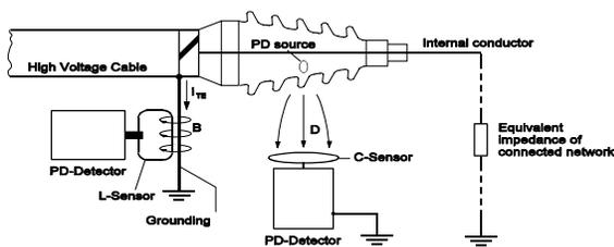
Figure 2: Field sensors for PD decoupling on cable terminations (rotating machines)
