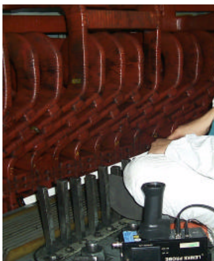
Figure 1: Inductive field coupling for location of PD affected coils in a hydro generator
