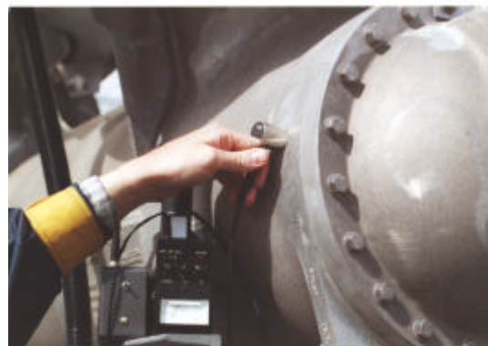
Figure 7: PD measurement on a gas-insulated substation using piezo electrical, acoustical measurement in connection with the PD probe LDP-5
