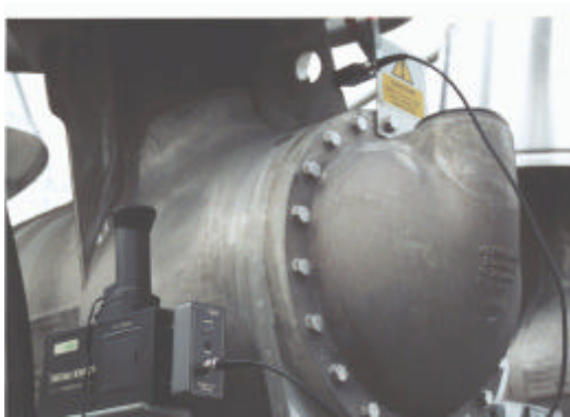
Figure 3b: UHF sensor applied to decouple PD from a high voltage GIS terminal
