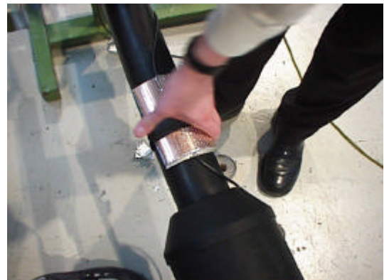
Figure 4a: DCD Directional Coupler Measuring System LDY-724; installation of a coupling sensor
