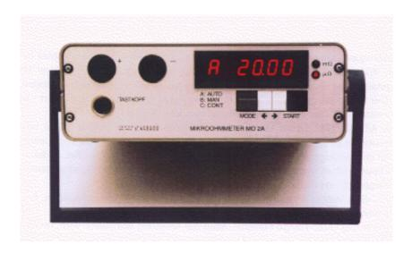
The MO 2A is used for measurement of connection resistance. The measurement procedure is based on a four-wire configuration with voltage/current measurement followed by calculation and display of the resistance value. During the measurement a DC pulsed current of approx. 20 Amperes is injected into the measurement object. Appropriate control of the measurement process by means of an embedded micro-controller eliminates error due to external offset voltages (e.g. thermal emf).
