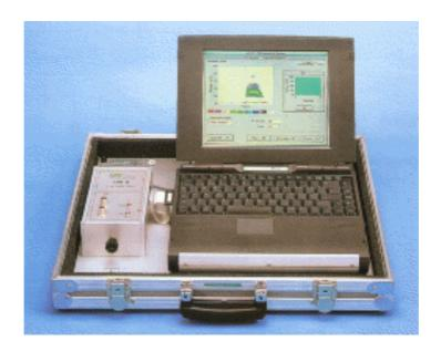
The measuring system LDS-5 is designed for computer-aided monitoring, recording and analysis of PD pulses detected by high voltage equipment using either the standardized coupling mode or the non-conventional field coupling mode.
