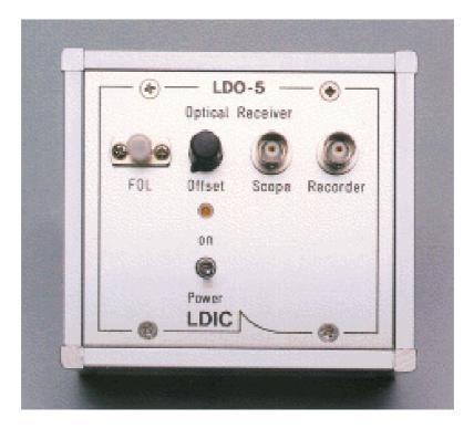
The Optic Receiver LDO-5 is applicable for potential-free signal transmission from the DIFFERENTIAL LEMKE PROBE LDP-5 to the scope for monitoring PD events. It converts the optical signals derived from the LDP-5/BOA into electrical signals useable for post-processing with an additional scope or a XY-recorder.
