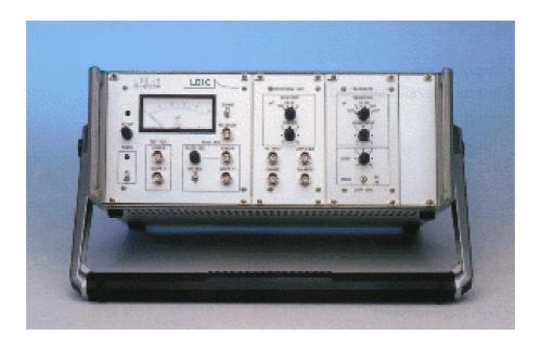
The PD detector LDD-5 is designed for standardized measurements according to IEC 60270. This new development of LDIC bases on large experience in wide band PD measuring technique. The main fields of application of the LDD-5 are PD quality tests on HV equipment and fundamental PD studies in research and education.
