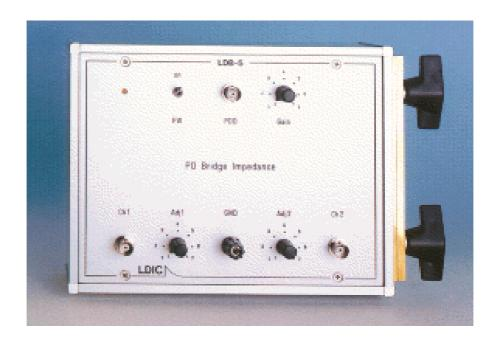
The bridge impedance LDB-5 serves for the design of the bridge circuit according to IEC 60270 or DIN VDE 0434, respectively.
